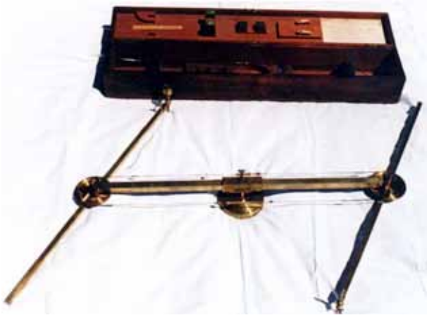
Wallace's Eidograph, a device for scaling down drawings and maps, etc.
